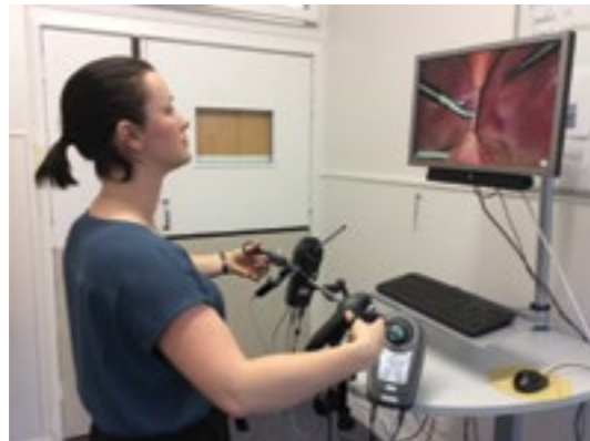
Figure 3. Monitor in suboptimal position, resulting in upward angle of gaze and somewhat forward head position.
